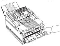
5. Insert a sheet of paper face up, adjusting the guides again to ensure the paper is straight.
